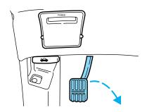
The BRAKE warning lamp in the instrument cluster illuminates and remains illuminated (when the ignition is turned ON) until the parking brake is released.
